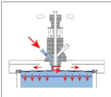
**Figure 3. Cross-section of the nozzle valve and flow distribution system.**
